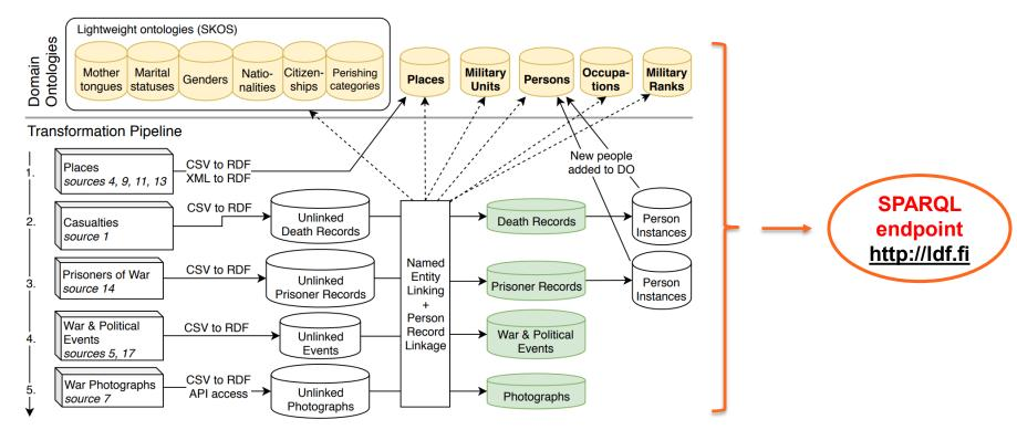
Figure 3. The 5-step WarSampo data transformation process. Dashed arrows represent entity linking, while solid arrows convey data flow.
